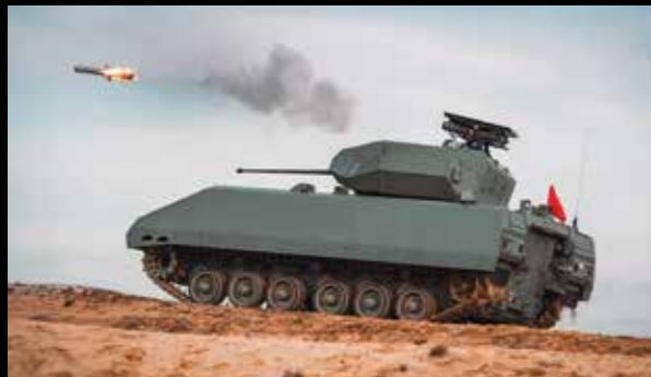
The Hunter AFV is Singapore's first fully digitalised platform and is equipped with a remote-controlled weapon system, a 30mm cannon, anti-tank guided missiles, an integrated combat cockpit and enhanced capabilities. The Hunter AFV enables its crew to engage threats with speed and precision.
