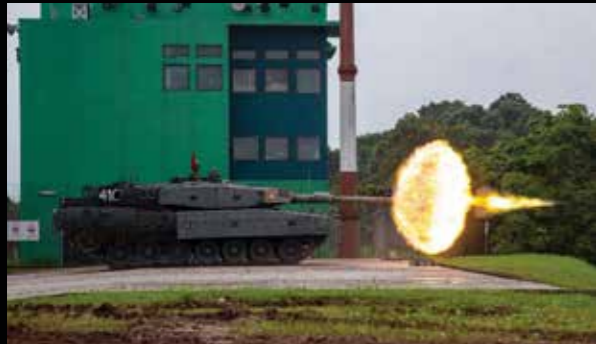
The Leopard 2SG (L2SG) Main Battle Tank combines superior firepower, mobility and protection. It is equipped with a 120mm smoothbore gun and stabilised fire control system capable of delivering precise and devastating firepower.
